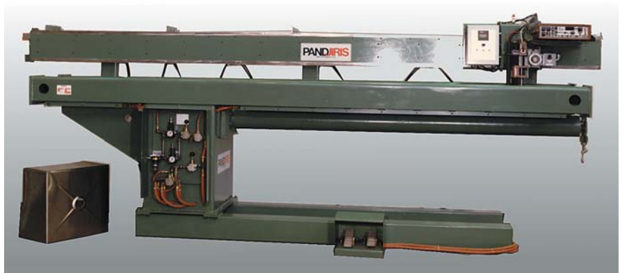
Double-ended seamer for flat sheet and corner welding of stainless steel sinks
