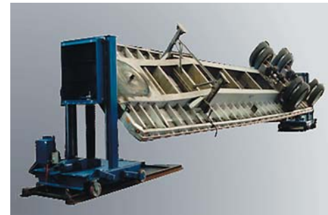
Power Elevating Head & Tail Stock
