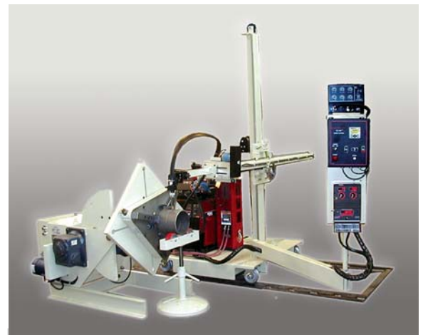
Delta MIG Pipe Welding System
