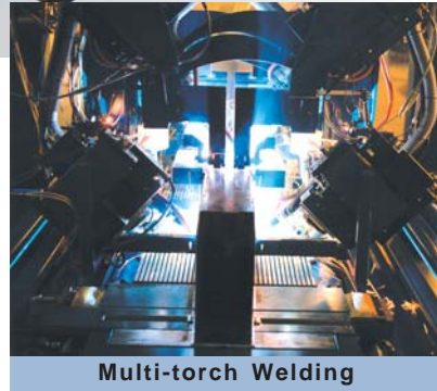
Touch Screen PLC Control with Video Monitoring of Four Torches
