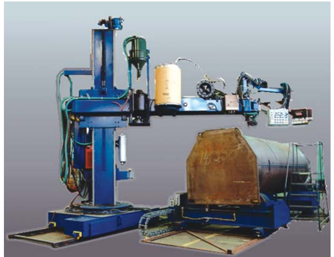
Special 1400 Series Manipulator for Longitudinal & Circumferential Welding
