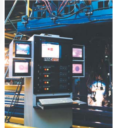
Touch Screen PLC Control with Video Monitoring of Four Torches
