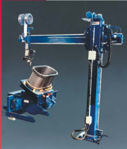
Elliptical Welding System with PLC Multi-Axis Controller
