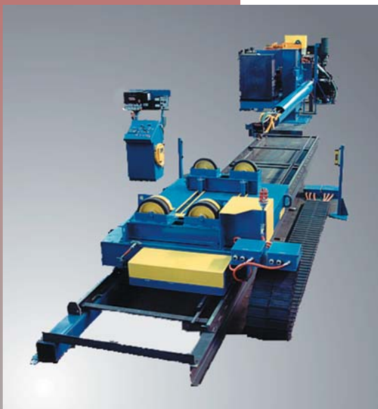
Small ID Internal/External Longitudinal Seam Welder with Tandem SAW
