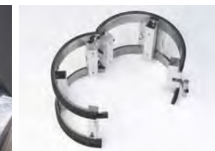
Guide Rings Mount Head on Pipe
